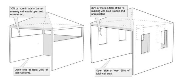
Rectangular areas have been used in the above diagrams; the same principles apply to any other shaped area.
