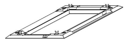
Line up the hooks with the receptacles on the IO1000, and gently push the fascia into position. The switch should be on the right hand side of the fire. The angle of the hooks can be adjusted if necessary to ensure a good fit.
