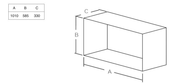
Where possible, it is recommended that the cavity is made slightly larger than the above dimensions to give the installer the maximum amount of space to work in.
