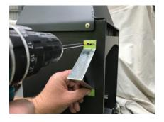
The large standoffs are screwed on the sides. The standoffs are placed at the opposite corners.
